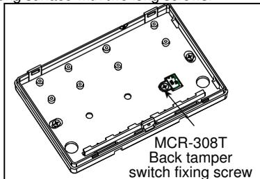
forcibly removed from its mounting place, the actuator breaks away from the base, causing the tamper switch opening - a tamper alarm is consequently transmitted.
