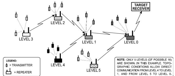
Figure 2. Multi-Level Repeater Configuration
