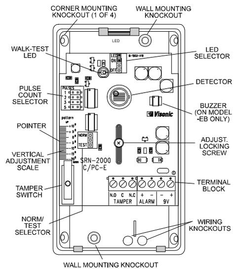
Figure 9. SRN-2000C/PC-E and -EB, Inside View
