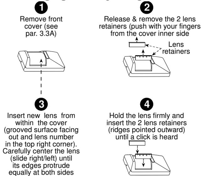
Figure 2. Changing and Adjusting Lens
