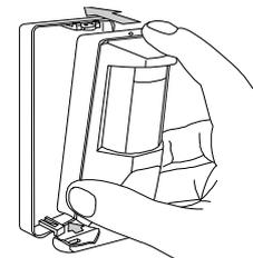
Figure 4. Replacing the Cover
