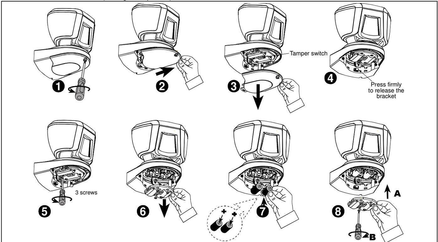
**Figure 3 - Battery Insertion**
